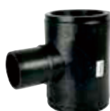
Reducer Tee SDR 11 PE 100 Gas : 10 Bar / Water : 16 Bar
