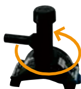
Tapping Tee with 360° Rotating Outlet SDR 11 PE 100 Gas : 10 Bar / Water : 16 Bar
