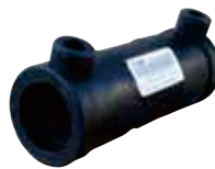
Coupler (Long) SDR 11 PE 100 Gas : 10 Bar / Water : 16 Bar
