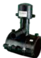
Tapping Tee with End Cap SDR 11 PE 100 Gas : 10 Bar / Water : 16 Bar
